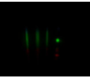
**Picture 24**The blue film seems to contain anti-green and anti-red dye.
