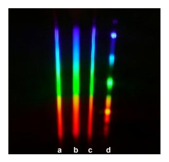
Lamps such as a, b and c generate light by heating a filament of wound metal wire and their optical fingerprints<sup>6</sup> are continuous. Lamps such as d generate light due to gas excitation and their optical fingerprints are non continuous. It is therefore clear that inspecting the optical fingerprints of the lamps, we can deduce which category they belong<sup>7</sup>.
