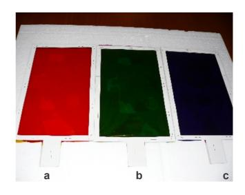
**Picture 22**The red film seems to contain anti-blue and anti-green dye<sup>10</sup>.
