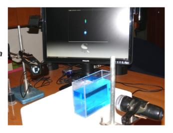
Using a simple spectroscopic device adapted to a webcamera, we can go a bit deeper in the perception of color.
