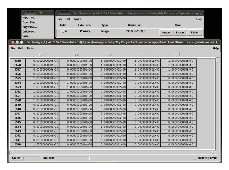
Each table cell represents a pixel of image of spectrum and its value corresponds to the light intensity in that point in an arbitrary way.
